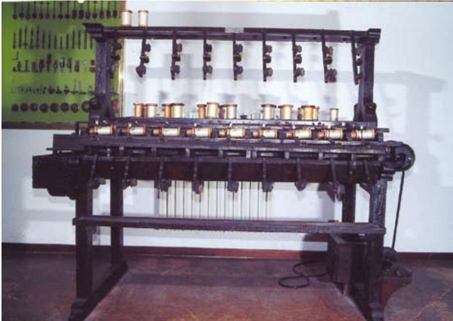
Machine for twisting, or «throwing», the silk filaments.
